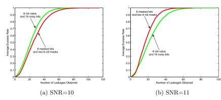
Fig. 12: Avg. success rate of an 8-bit  $3^{rd}$  order masking scheme with noisy counterpart.
