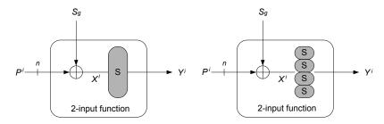
Fig. 2: Single block and multiple block cipher implementation.
