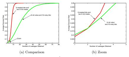
Fig. 11: Avg. success rate of an 8-bit  $3^{rd}$  order masking scheme with noisy counterpart.
