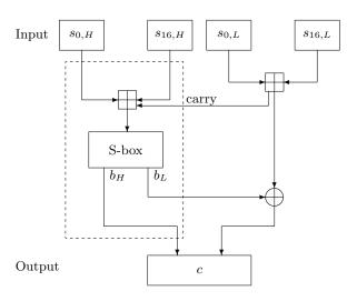
Fig. 3. A reconstructed block for the modular addition and S-box
