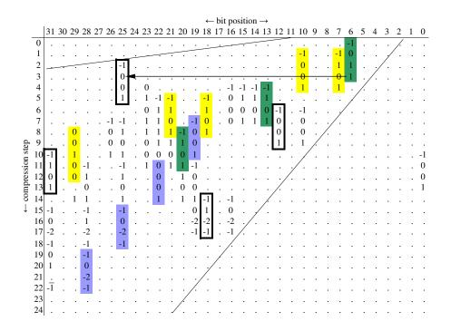
**Fig. 3.** In our path, differences and conditions are spread by introducing a *dispersion* difference in step i = 3 which has a high rotation value ( $s_3 = 19$ ). This dispersion difference causes new conditions, which are marked by a box in this figure. Because of introducing a new difference, the number of conditions is higher (146). However, no contradictions appear.
